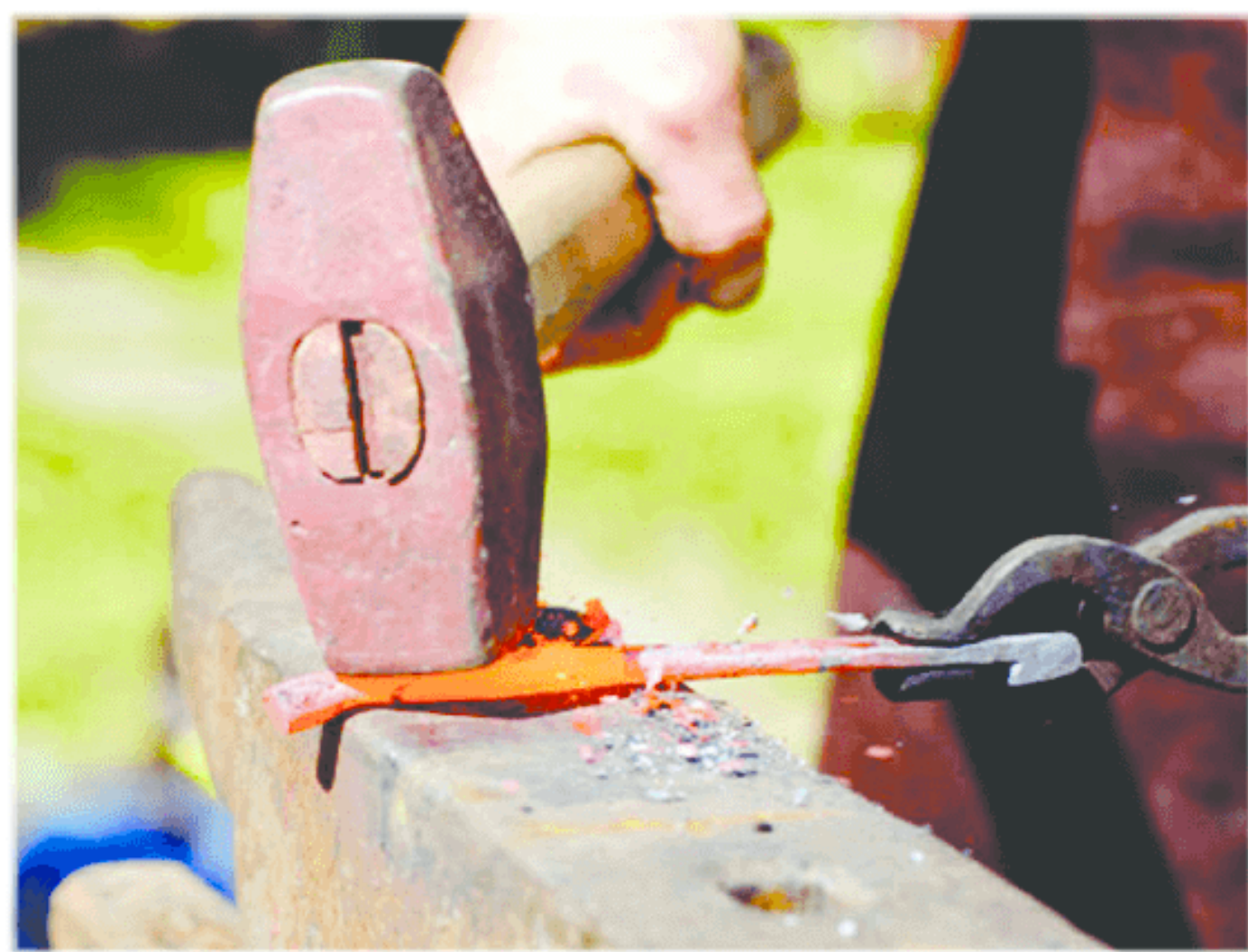
FIGURE 1 Malleable and ductile substances are those that dent or stretch when a force is applied and can be drawn into wires. By contrast, a brittle substance will crack and shatter under the same conditions.
