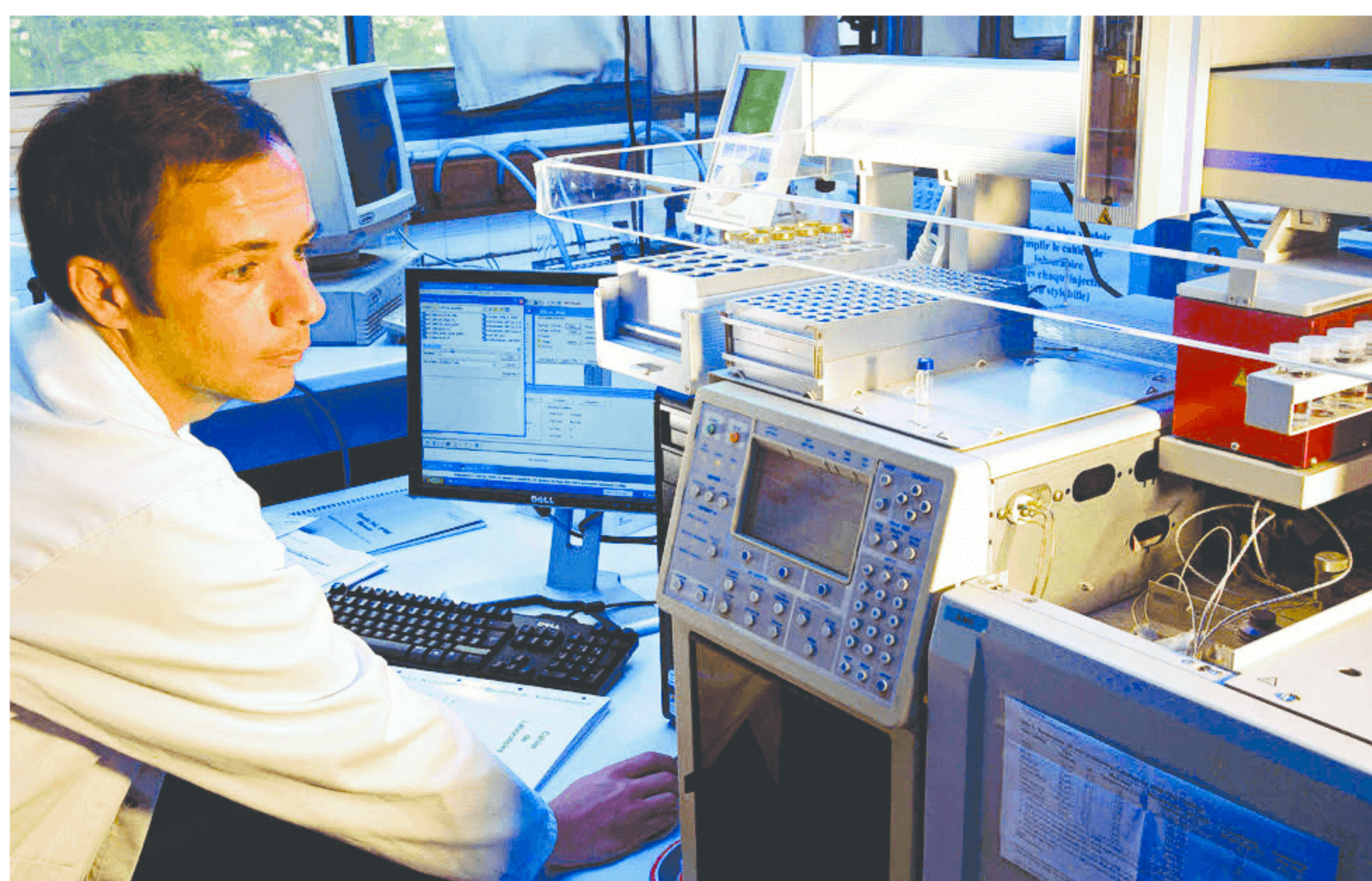
FIGURE 1 This researcher is using gas chromatography to analyse samples of wine to determine the aromatic characteristics of different grapes and their suitability for use in winemaking.
