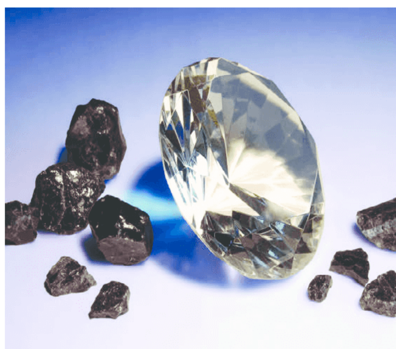
FIGURE 13 Diamond and graphite (black lumps) both consist of pure carbon . Their vastly different properties are caused by the different arrangement of covalently bonded carbon atoms. Different forms of the same element like these are known as allotropes .
