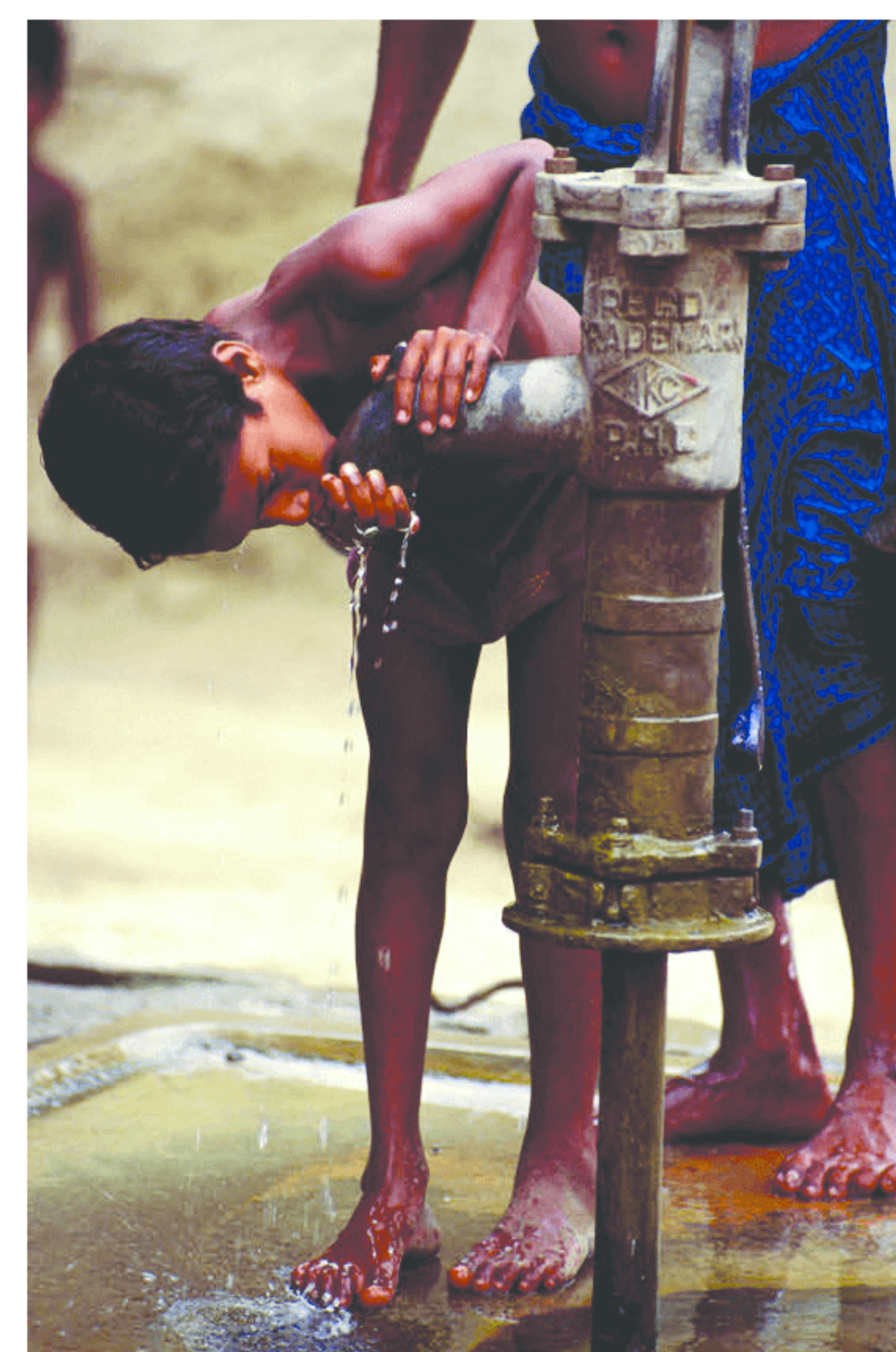
FIGURE 22 Wells like this shallow tube well became a very important water source in Bangladesh from the late twentieth century. This followed an extensive shallow tube well drinking water program intended to provide villagers a bacteria free water supply for drinking washing and agriculture. Unfortunately authorities did not test for arsenic in the groundwater and it is now known that many of these shallow wells are heavily contaminated with naturally occurring arsenic. Similar problems are known to occur in many parts of Southeast Asia , where similar hydrology results in high concentrations of arsenic in near surface groundwater.
