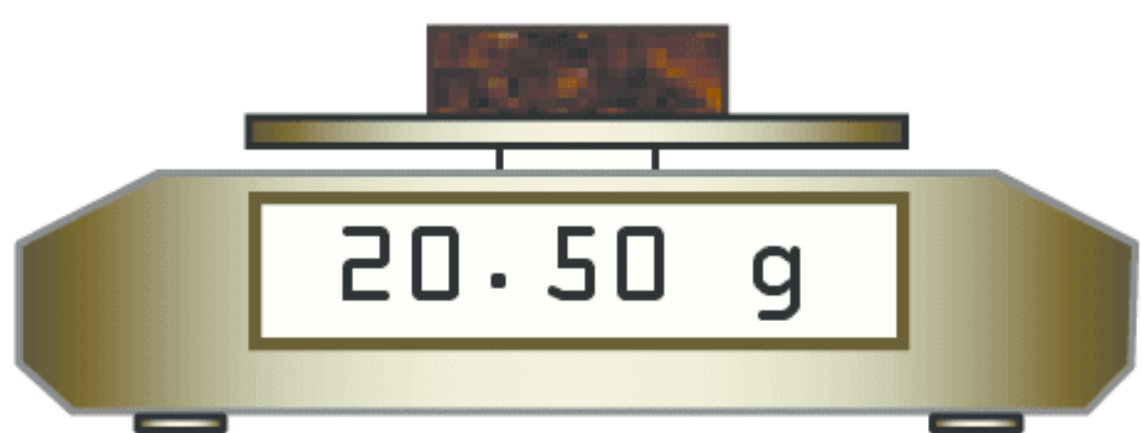
FIGURE 7 The last digit of a digital display has some uncertainty, you will sometimes see the value of this digit fluctuate. The measurement shown here is written as 20.50 g rather than 20.5 g. Recording the zero better reflects the precision offered by the instrument.
