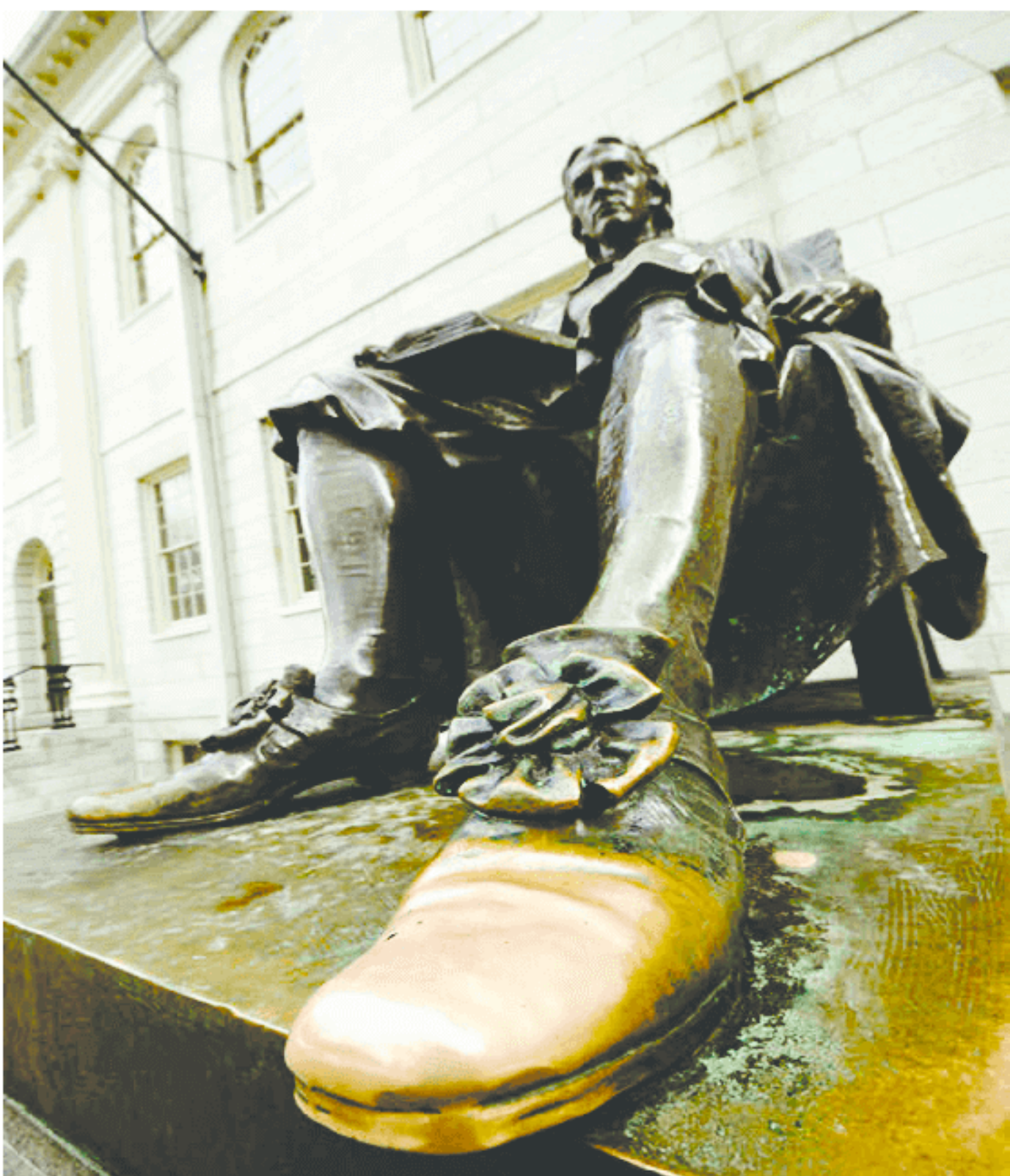
FIGURE 1 The alloy bronze , used in this statue is an homogeneous mixture of copper and tin . Use of bronze is believed to date to at least the 4th millennium B.C. It was one of the most important materials used by early civilisations. Much harder than pure copper or stone, it was used for tools, weapons, decorative plaques and statues. The melting point of bronze, like that of all mixtures, is not fixed or well defined but depends upon several factors including the % composition of the bronze. (See table.)
