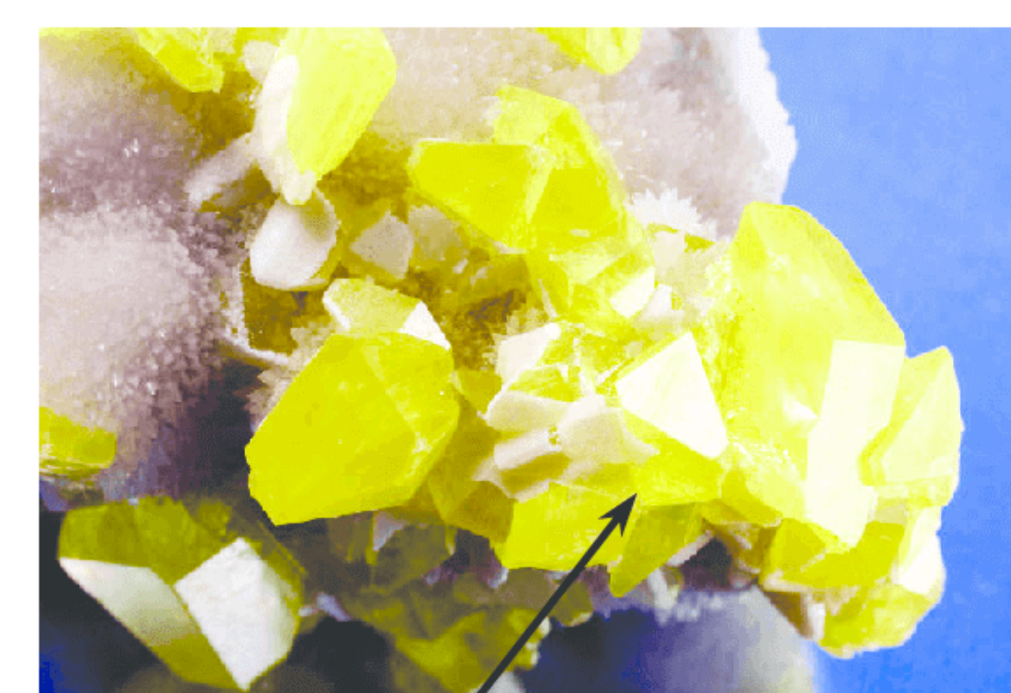
FIGURE 6 It must be noted that some of the non-metal elements exist in a variety of allotropic forms with different molecular structures other than those listed here. Oxygen for example normally occurs as \text{O}_2 however, it also exists as ozone, \text{O}_3 . The yellow, solid form of sulfur commonly used in the laboratory is rhombic sulfur which consists of puckered \text{S}_8 rings of sulfur atoms.
